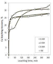
Fig. 4. Effect of ammonia ions concentration on Cu recovery; s/l = 1:10, initial  $S_2O_3^{2-}$ concentration 1.0 mol/dm<sup>3</sup>, temperature 25 °C
