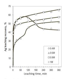
Fig. 1. Effect of thiosulfate ions concentration on Ag recovery; s/l = 1:10, initial NH<sub>3</sub> concentration 0.6 mol/dm<sup>3</sup>, temperature 25 °C
