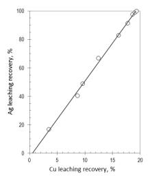
Fig. 10. Ag recovery vs. Cu recovery in thiosulfate leaching after modification with NaOH; s/l = 1:10, initial NH<sub>3</sub> concentration 0.8 mol/dm<sup>3</sup>, initial S<sub>2</sub>O<sub>3</sub><sup>2-</sup> concentration 1.0 mol/dm<sup>3</sup>, temperature 25 °C
