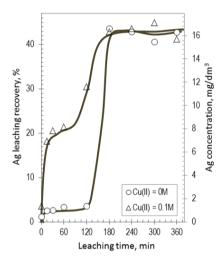
Fig. 5. Effect of addition of Cu(II) on Ag recovery; s/l = 1:10, initial NH<sub>3</sub> concentration 0.6 mol/dm<sup>3</sup>, initial S<sub>2</sub>O<sub>3</sub><sup>2-</sup> concentration 0.5 mol/dm<sup>3</sup>, temperature 25 °C
