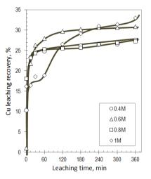
Fig. 2. Effect of thiosulfate ions concentration on Cu recovery; s/l = 1:10, initial NH<sub>3</sub> concentration 0.6 mol/dm<sup>3</sup>, temperature 25 °C
