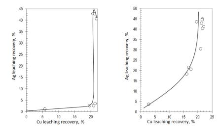
Fig. 6. Ag recovery vs. Cu recovery in thiosulfate leaching without addition of Cu(II) ions; s/l = 1:10, initial NH<sub>3</sub> concentration 0.6 mol/dm<sup>3</sup>, initial S<sub>2</sub>O<sub>3</sub><sup>2-</sup> concentration 0.5 mol/dm<sup>3</sup>, temperature 25 °C
